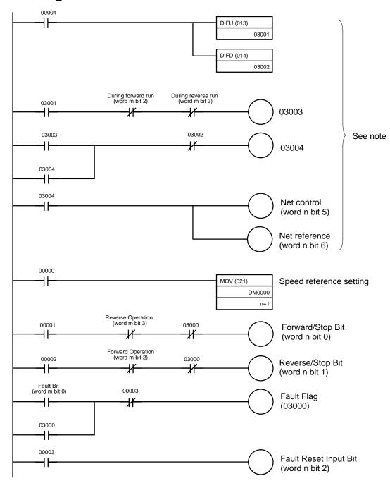
**Note** This program is not required if the b1-01 (Frequency Reference Selection) and b1-02 (Inverter Run Command Selection) are set to "3."
